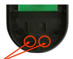
Prepared Pre-punched holes for cables,
